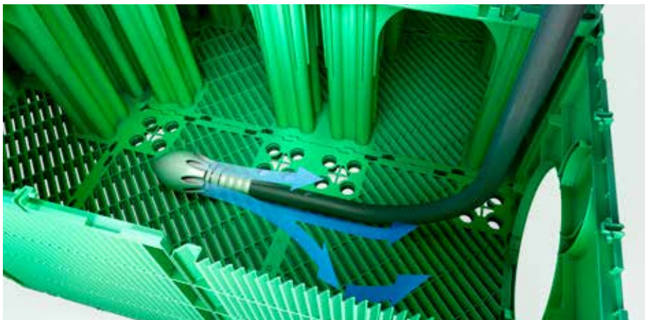
Innovative construction of side panels and bottom plates - inclined ribbing, which during cleaning reverts the pressure water jet and prevents damage to the geotextile
