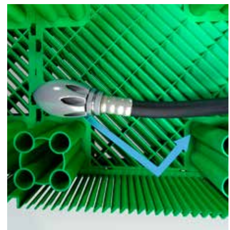
Innovative construction of side panels and bottom plates - inclined ribbing, which during cleaning reverts the pressure water jet and prevents damage to the geotextile
